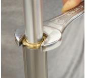
Using the 23mm open-end wrench, carefully turn the upper brass guide out of the cartridge. Make sure that the longitudinal guides of the cartridge are not in engagement with the open-end wrench and are therefore not damaged.
