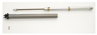
When both screws are loosened, the hydraulic gas spring can be pulled out of the cartridge.
