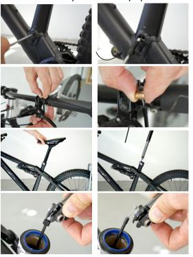
Unscrew the Postpin axis with a 5mm Allen key.
