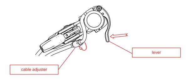
**Step 10:** Cut the protruding Bowden cable within the lever length using a cable cutter.
