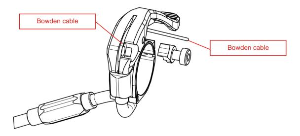
**Step 8:** Position the clamping jaw over the Bowden cable and partially screw in the clamping screw. Ensure that the lever is in the NOT-pressed position. Tighten the clamping screw under slight tension on the Bowden cable to 1,5 Nm.
