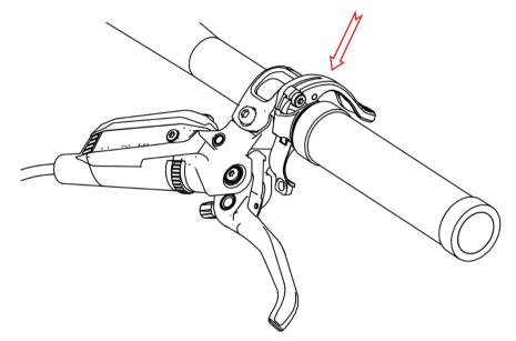
Tip: With the clamping part open, find the desired position by placing your hand on the grip in the riding position. Place your thumb on the "pressure area" of the lever to determine the perfect position. In the illustrated case, the clamping position of the Remote is between the grip and the brake lever.
