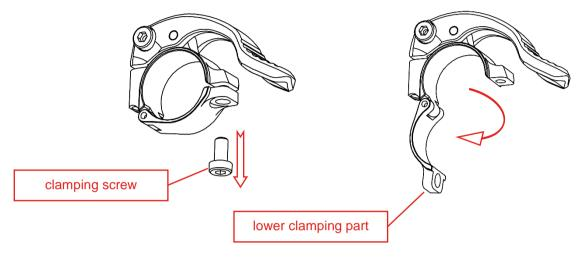
Step 1: Open the clamping screw with a 3mm Hex key and fully release the lower clamping part.
